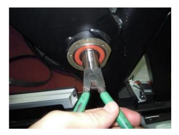
4. Install the snap ring (item #5 in the table) to secure the bearing on the left side of the frame.
