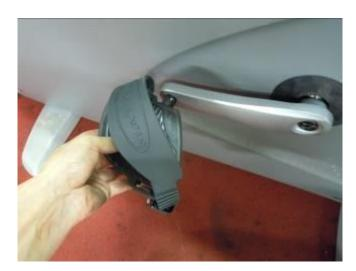
11. Use a pedal wrench to attach the pedals (item #9 in the table).
