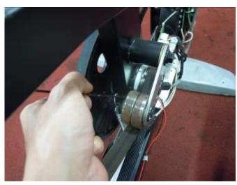
7. Use a hook or loop of wire to install the spring on the frame.
