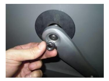
9. Using a Hexagon-Socket-Head sleeve wrench, install the washer (item #6 in the table) and nut (item #7 in the table) to hold the crank (item #2 & #3 in the table) to the pedal axle set. **NOTE:** Torque the nut to 80 N-m/800 kgf-cm.
